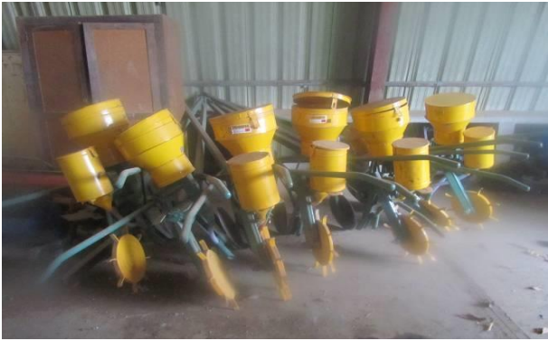
Figure 8: Locally made animal drawn direct seeder by Nandra Engineering Moshi
