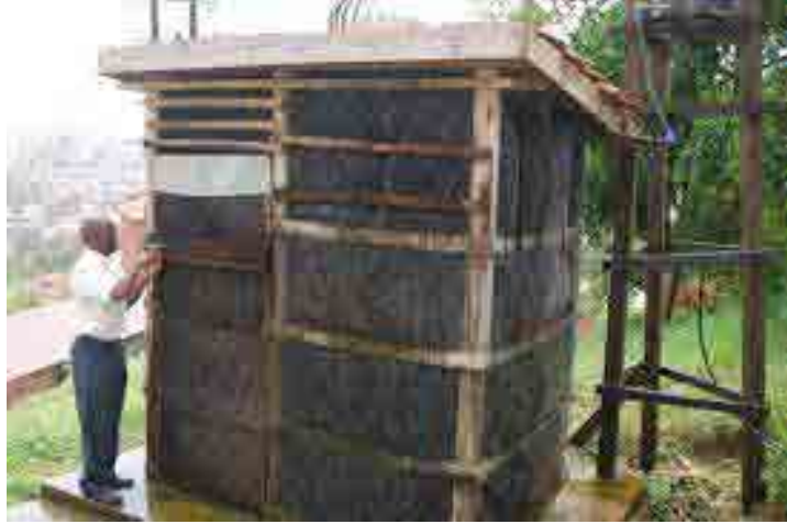
Kielelezo Na 15: Jokofu la mkaa (Charcoal cooler - CC)
